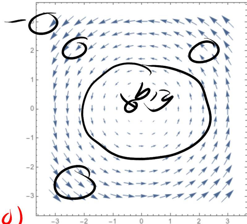
$$\nabla \times \vec{F}(x, y) = \frac{\partial F_2}{\partial x} - \frac{\partial F_1}{\partial y}$$
